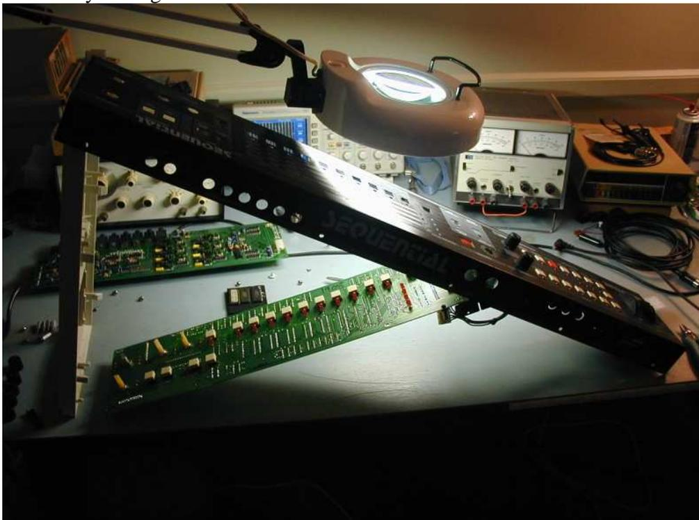
After I did it this way, I decided that probably removing both the digital board and the power supply board would have been easier. I will leave that up to you.
