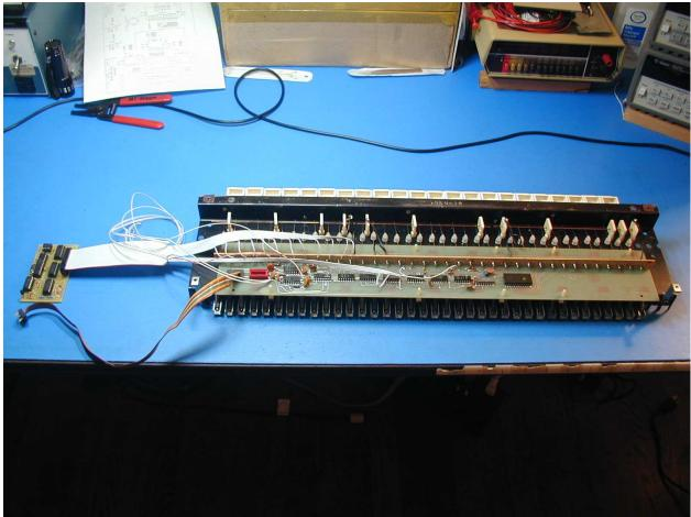
3) Pin 1 of the connector connects to the wire with the red stripe on it. Pin 2 connects to the next wire, and so on. There are 26 wires in all. Three signals appear twice in the cable, at each end: +5V, ground, and -15V. Use both wires for these signals, twisting the ends together after you have stripped off the insulation.
