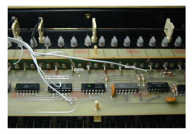
7) Solder the +5V and ground wires (two each, with the ends twisted together) onto the appropriate pcb traces, as shown in a previous photo.
