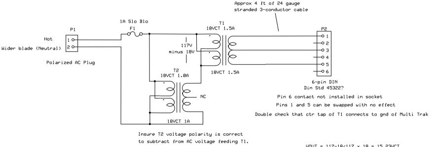
Transformers were purchased at MPJA.com When connecting primaries in parallel for 110V, don't connect a lead with a dot to a lead without it.  $VOUT = 117-18/117 \times 18 = 15.23VCT$
